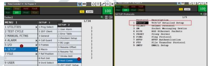
Figure 4. Fanuc Protocol setup
